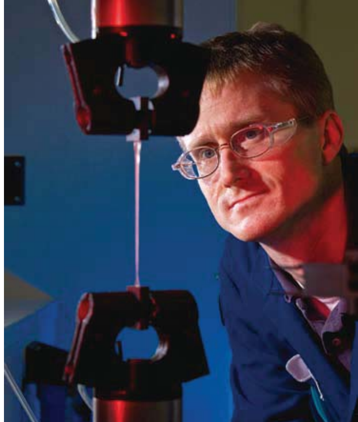
Andy Winesett, senior physicist, tests the tensile strength of a polymer sample. The rate at which it stretches and the force required to break it are important measures of polymer performance.
